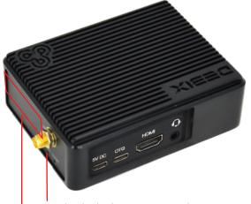
Circular hole for an external Wi-Fi antenna Square hole to prevent Wi-Fi signal blocking
